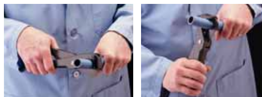
The rotating/rocking technique produces fast easy cuts.
