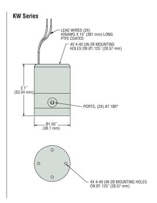
$\hbox{3-Way, Normally Closed (N.C.), Multi-Purpose, Directional Control}\\$
