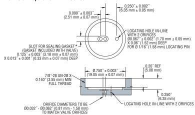
Note: Valve spacing to be 1.00" (25.4 mm) min. center to center \*FFKM gasket is provided for manifold mount valves.
