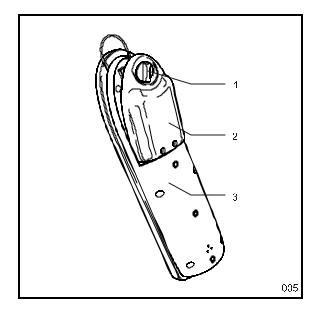
$\Rightarrow$  Insert the charged battery [2] into the transmitter [3] (the transmitter should point downwards),
