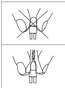
**Halogen Lamp Warning!** This fixture is fitted with halogen lamps which are highly susceptible to damage if improperly handled. Never touch the lamps with your bare fingers as the oil from your hands will shorten lamp life. Also, never move the fixture until the lamps have had ample time to cool. Remember, lamps are not covered under warranty conditions.
