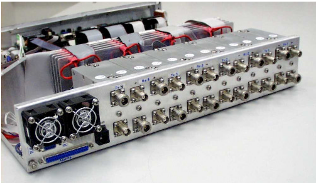
Figure 11: Bias-T inputs / outputs and numbering
