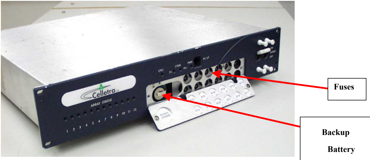
Figure 9: Fuse and backup battery location
