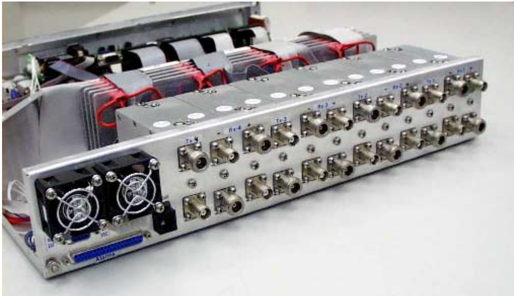
Figure 11: Bias-T inputs / outputs and numbering
