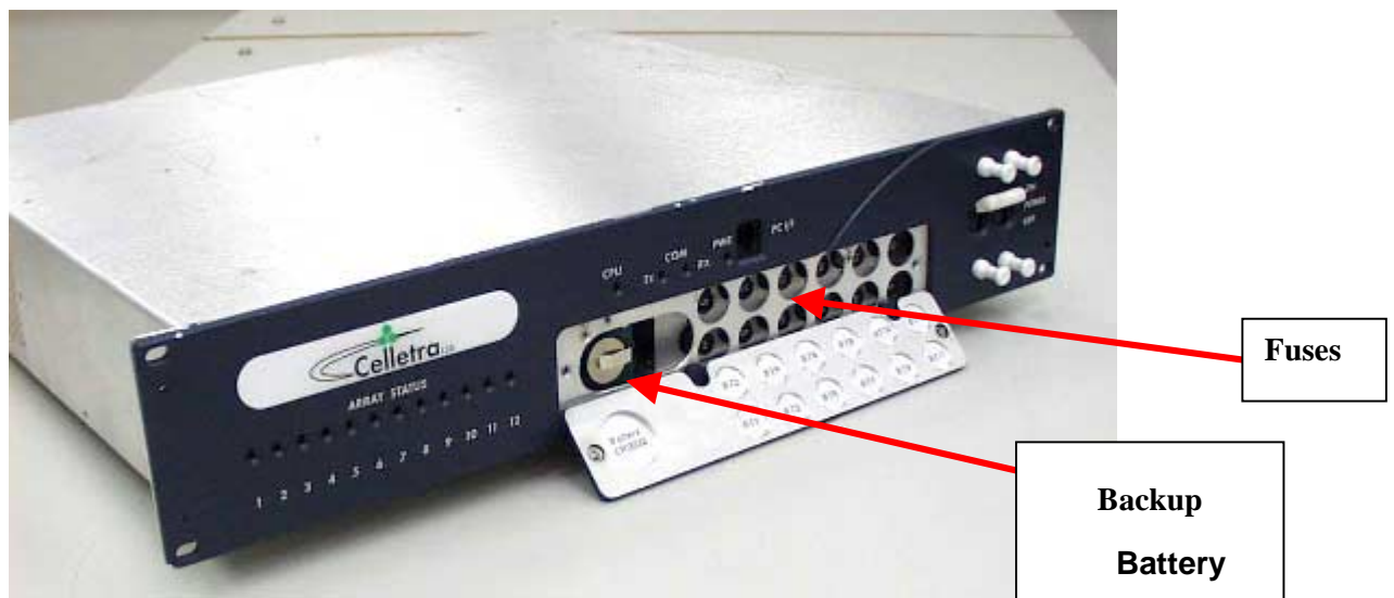
Figure 9: Fuse and backup battery location
