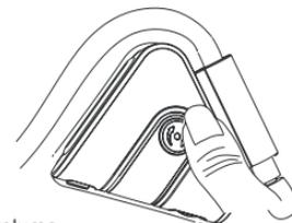
2. Press the Volume control button to adjust the volume.
