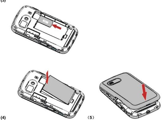
Note: make sure that the metallic contacts of the battery are facing the metallic contacts inside the battery slot.
