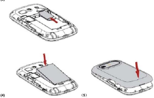
Note: make sure that the metallic contacts of the battery are facing the metallic contacts inside the battery slot.
