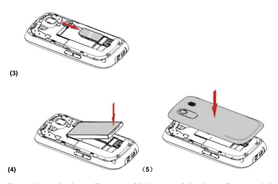
Note: make sure that the metallic contacts of the battery are facing the metallic contacts in the battery slot.
