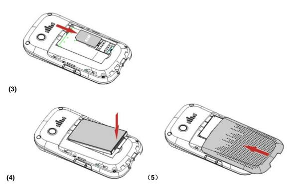
Note: make sure that the metallic contacts of the battery are facing the metallic contacts in the battery slot.
