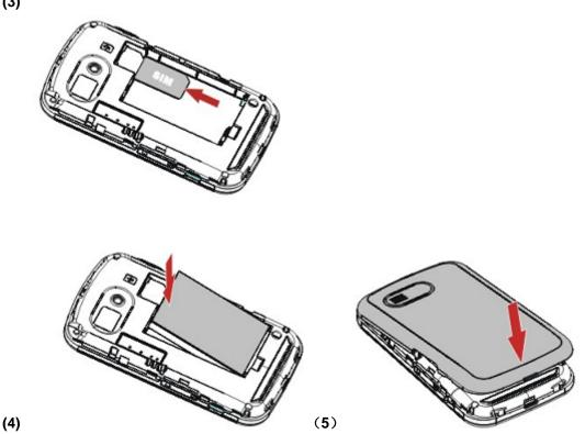
Note: make sure that the metallic contacts of the battery are facing the metallic contacts in the battery slot.
