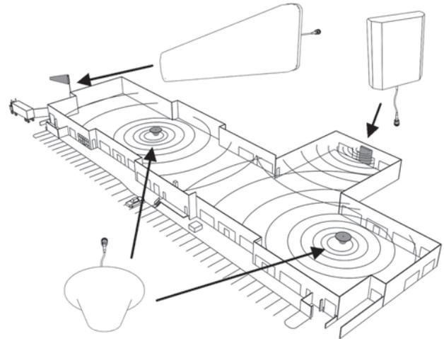
Keep in mind that floor structures in multistory buildings can cause significant signal loss, which means that you may need to install interior antennas on more than one floor. Here is an example of a multistory installation:
