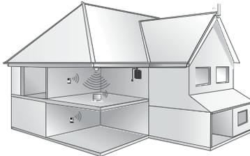
2. Using the CM240 or CM400 cable, connect the inside antenna to the booster connector marked **INSIDE** (see page 4).
