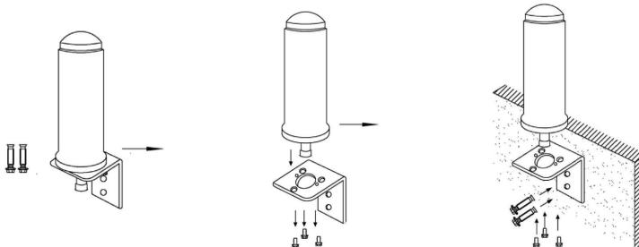
**Note:** If desired surface for installation plate is wood or concrete, wood or masonry screws for L-plate will have to be purchased separately.
