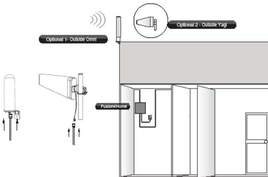
**IMPORTANT:** For boosters enhancing T-Mobile's AWS frequencies, the FCC has stated for consumer signal boosters operating as a fixed station in the 1710 - 1755 MHz uplink 2110 - 2155 downlink bands, the users or installation manual must contain the 30 foot height restriction requirements per FCC 27.50(d)(4).
