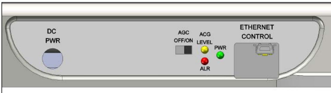
Figure 17: Repeater control panel
