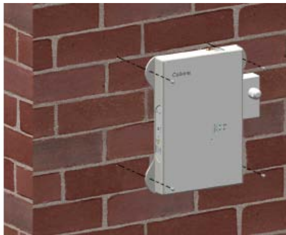
Figure 14: Repeater wall installation
