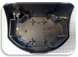
**Step 2** – Attach monitor assembly with 4 provided screws. Attach switch wires to dry contact junction.
