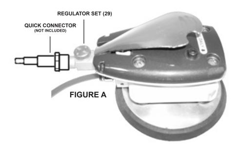
For best tool performance, you should incorporate an oiler, regulator, and in-line water filter as shown in the illustration on the next page.
