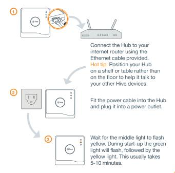
Once the yellow light is flashing, the Hub is set up and you can move onto installing the thermostat. If no lights are displayed immediately after the Hub has been turned on, check all cables are connected, the power outlet works and that you have connection. If the problem still persists, contact Hive Technical Support.
