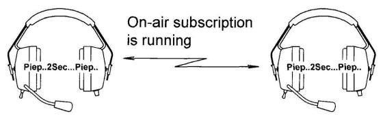
After approx. 30 seconds a high double-beep tone can be heard in both headsets. Two low tones before the high double-beep tone signalize an incorrect subscription. Start the on-air subscription procedure again.
