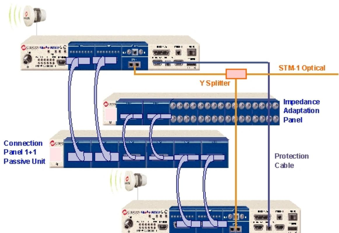
Figure 7-11 Protected Y Splitter Configuration for Unbalanced E1s
