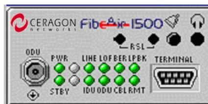
Figure 7-7 Slave LEDs
