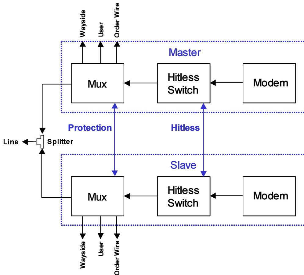
A special proprietary algorithm determines which ODU is transmitting error-free data. The error-free data is then passed on by the master switch in the IDU to the network.
