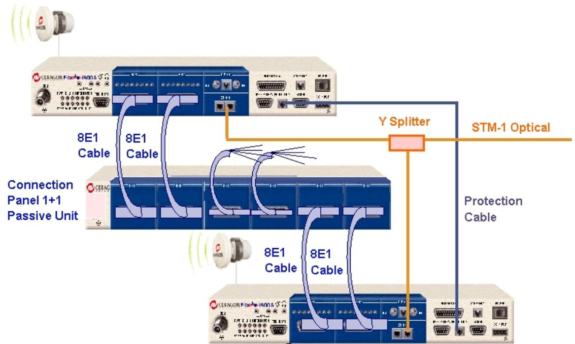
Figure 7-10 FibeAir 1500A/1528A Protected Configuration using Y Splitter
