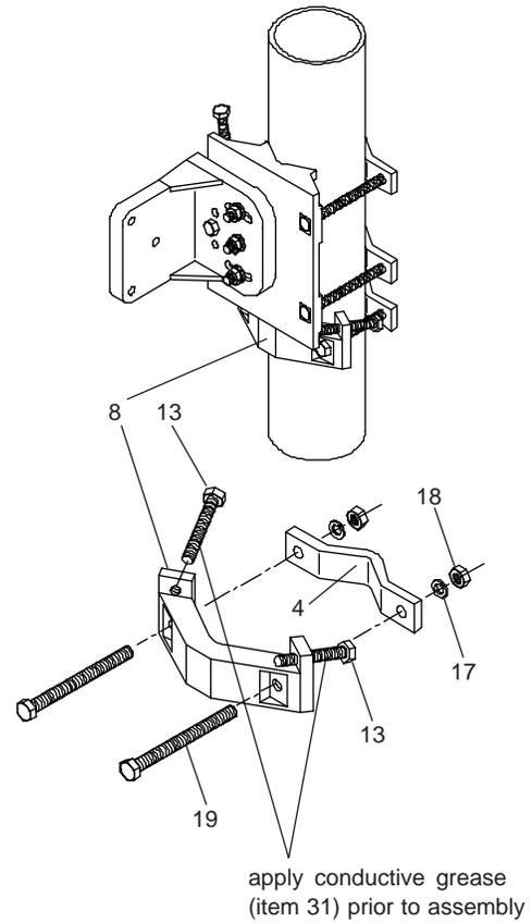
apply conductive grease (item 31) prior to assembly
