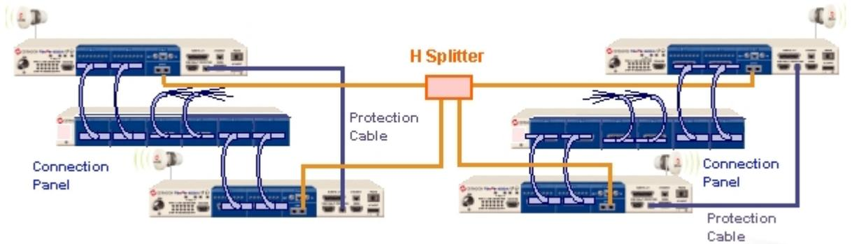
Figure 7-12 FibeAir 1500A/1528A Protected Configuration using H Splitter
