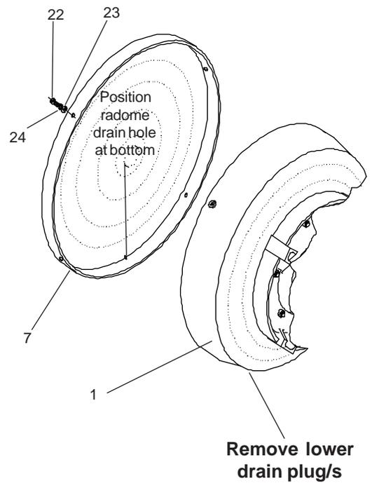
Remove lower drain plug/s
