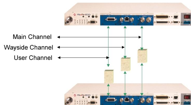
Figure 7-9 Splitter Connection
