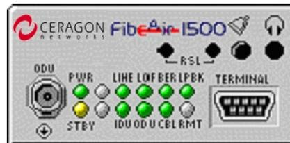
Figure 7-6 Master LEDs
