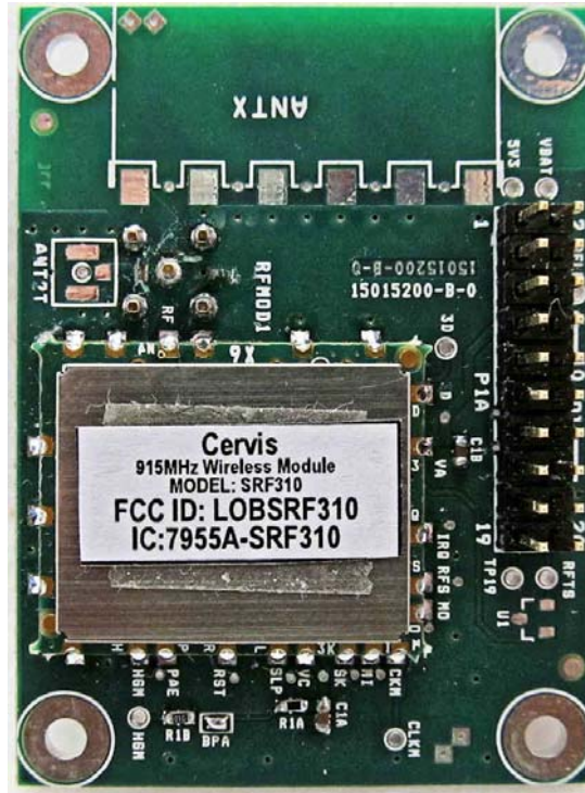
Figure 4. SRF310 installed in a typical host application.
