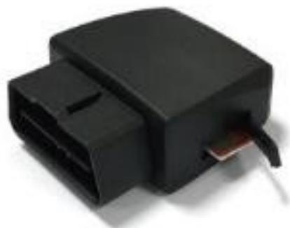
2. Insert 3G device into OBD port directly.
