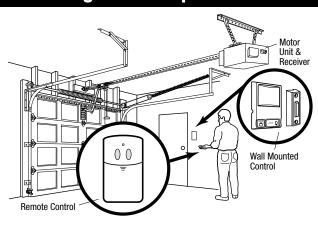
The clicker remote can be programmed to operate up to 2 garage door openers or gates. including different brands. All programming is done using the:
