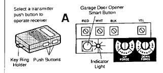
Make sure all transmitters are set to matching code switch positions as described above. Decide which transmitter push button you want to use to operate the opener.
