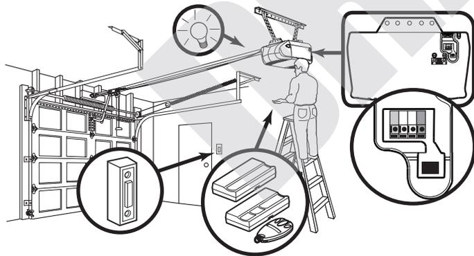
2. Press and release the “learn” button on the motor unit. The learn indicator light will glow steadily for 30 seconds.
