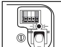
3. Within 30 seconds, press and hold the button on the 315MHz hand-held remote that you wish to operate your garage door.
