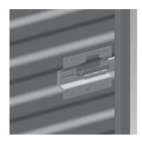
3. Position the overlock device in the door groove with the door hasp. (A customer lock may be present on the unit if the unit is currently rented.)
