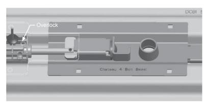
4. Slide the overlock toward the hasp until the end of the extended actuator touches the end of the hasp.
