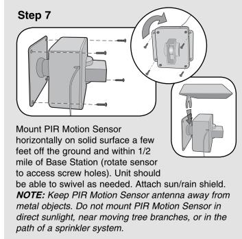
**Vehicle Alert Installation:** For cars, the best mounting position is about 4' high, between 10-20' back, and angled to see the back of car after passing the sensor.
