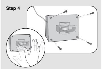
Test PIR Motion Sensor by waving hand in front of sensor. Test light should flash. Secure cover with the smallest screws.
