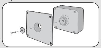
Attach PIR Motion Sensor box to mounting plate with large silver screw. Tighten screw until PIR Motion Sensor stays in place when repositioned.
