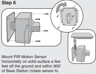
access screw holes). Unit should be able to swivel as needed. Attach sun/rain shield.
