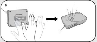
**B** Within 5 seconds, wave hand in front of PIR Motion Sensor. Test light will illuminate and Base Station will buzz.
