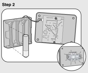
Install 4 AA Alkaline batteries (not provided). (Lithium batteries recommended for colder environments.) LED light will flash.
