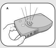
A Ensure Base Station and PIR Motion Sensor are in close proximity to each other. Press and release learn button on Base Station. Buzzer will sound.
