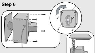
Mount PIR Motion Sensor horizontally on solid surface a few feet off the ground and within 1200'
