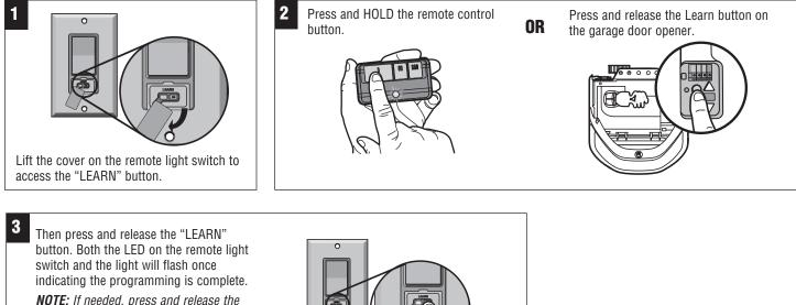
**NOTE:** If needed, press and release the "LEARN" button with a narrow instrument.
