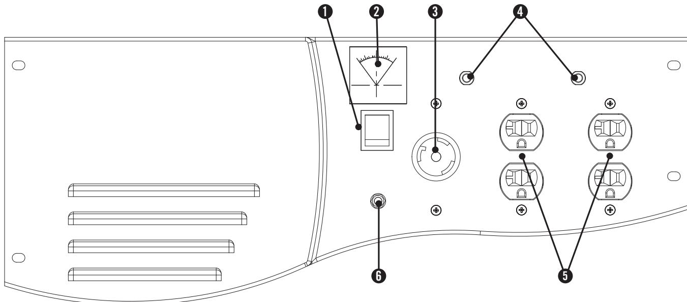
(1) **Engine Switch** – Flip the switch to the “On” position and pull the recoil starter to start the generator. Turn to the “Off” position to turn off the generator.
