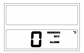
5.2.3 And then press **Alarm2** is to enter Min. setup mode (then with key tone), the Min. will be displayed as the below figure,
