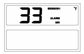
5.1.4 Press Alarm1 again under the above mode (then with key tone). The unit will be back to normal mode and display as the below figure,
