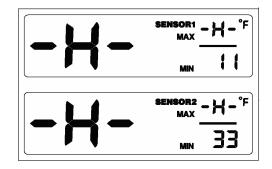
**4.4** When the temperature value is less than the Min limit -40 F, the unit will display as following,
