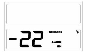
5.2.4 Press Alarm2 again under the above mode (then with key tone). The unit will be back to normal mode and display as the below figure.
