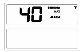
5.1.3 And then press Alarm1 is to enter Min. setup mode (then with key tone), the Min.
