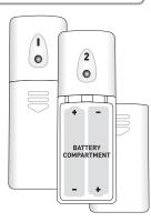
For the sensor that is placed in the freezer (#2), it is recommended that 2 "AA" lithium batteries be installed instead of alkaline batteries. Lithium batteries function at lower temperatures better than alkaline batteries.
