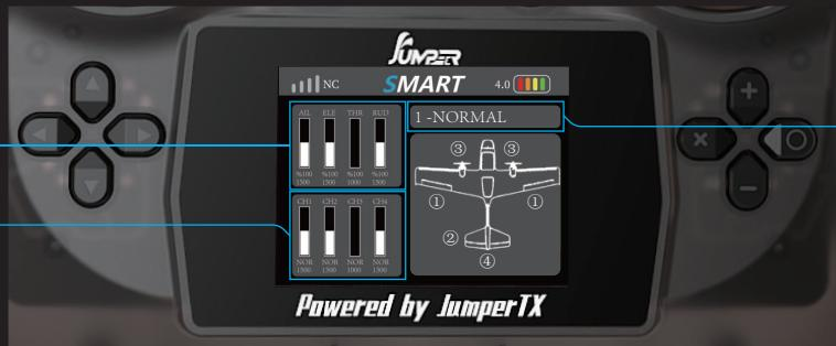
3. Press and hold the "O" button to enter the mixing settings. Use the left-side directional buttons (Up, Down, Left, Right) to set the direction (normal/reversed) and travel range for CH1-CH4. Press the "O" button again to toggle between normal and reversed direction. Use the "+" and "-" buttons to adjust the travel range. The "X" button exits.
