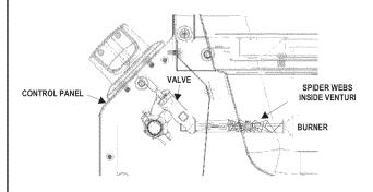
In some areas of the country, spiders or small insects have been known to create "flashback" problems. The spiders spin webs, build nests and lay eggs in the grill's venturi tube(s) obstructing the flow of gas to the burner. The backed-up gas can ignite in the venturi behind the control panel. This is known as a flashback and it can damage your grill and even cause injury.
