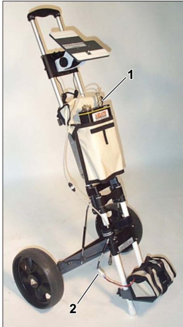
Fig. 4-4 – Battery and cabling support
