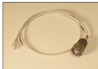
Inverted Network Cable
