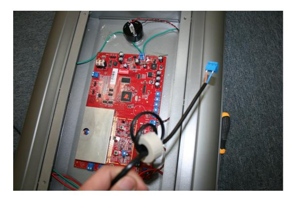
Step4: Make the other core around by 3-loop line at the other end of line.
