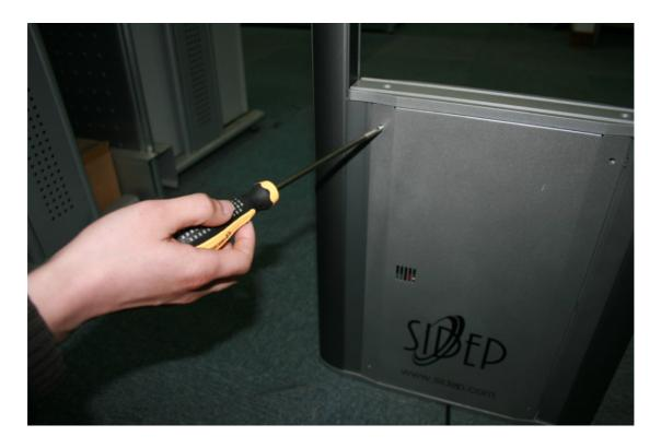
Step2: Screw the power line terminal (no positive and negative).
