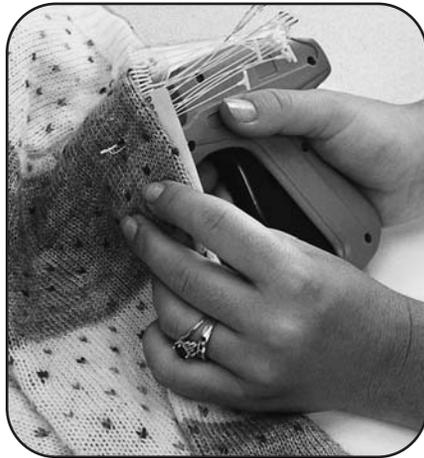
2. Line up the fastener gun needle with the hole. Push the needle through the fabric and the hole. Squeeze the trigger.
