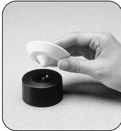
1. Place the plastic dome of the hard tag in the detacher well and push down on the pin, then gently lift the pin away from the detacher. For Designer and ChekInk II tags, place the fastener in the detacher well.
