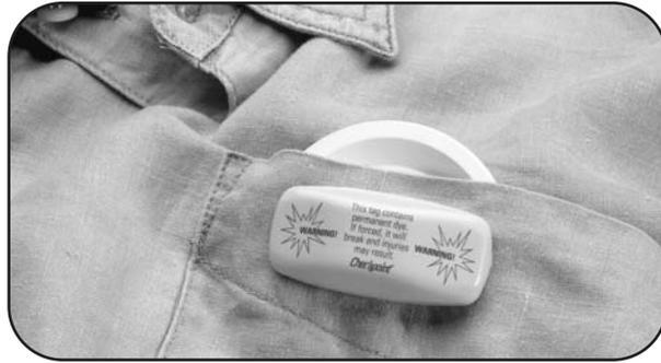
1. Holding the tag, push the pin through the item until it can be seen through the other side.
