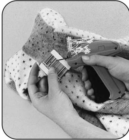
1. Attach the Flex Tag or hang tag with a Tagger, Mini Tach-It, Swiftach, Dennison Loop, or similar device, just as you do with pricing hang tags. Lay the Flex Tag flat against the item, with the hole where you want to attach the tag.
