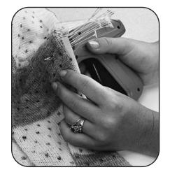
2. Line up the fastener gun needle with the hole. Push the needle through the fabric and the hole. Squeeze the trigger.
