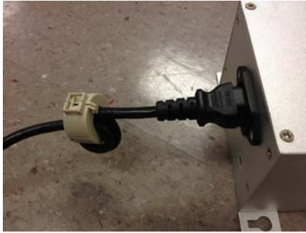
Figure 14.4 AC Power Cord Ferrite
