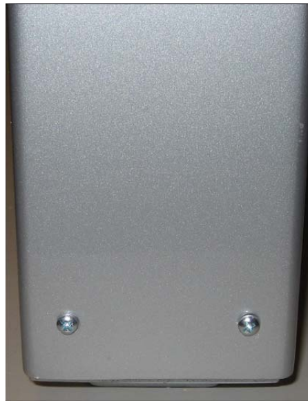
Figure 1.3 Bottom side screws removal
