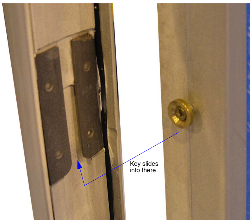
Figure 1.17 Sliding the frame side sections down
