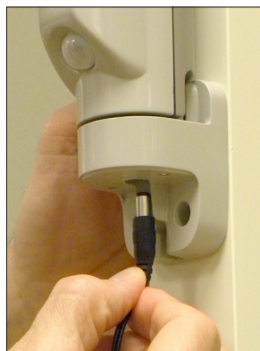
Figure 6 - Insert power supply cord as applicable
