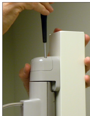
Figure 7 - Screw in both top and bottom Caps
