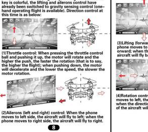
(3)Lifting (forward and backward) control: When phone moves to forward side, the aircraft will fly aircraft will fly backward moves to left, the nose of the aircraft will rotate to left when the direction control ball moves to right, the nose of the aircraft will rotate to right.
