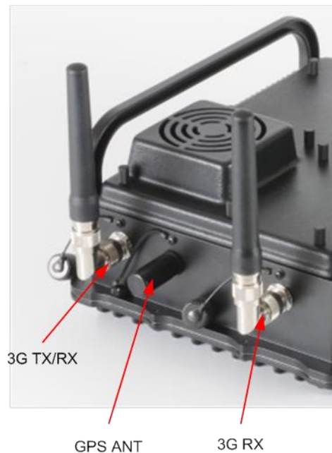
Figure 39 SMARTLINK BTS with Antennas connected
