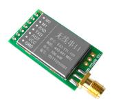
E32-TTL-100 is a wireless transceiver module with LoRa spread-spectrum technology, operates at 434MHz, based on original imported RFIC SX1278 from SEMTECH, transparent transmission is available, TTL level. The module adopts LoRa spread-spectrum technology, which means the transmitting distance is much longer than before. The advantages of this module is more concentrated power density and better anti-interference performance.
