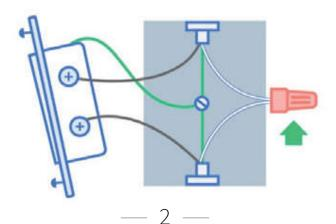
e) Unscrew the wires and connect them according to picture below.
