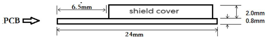
The following figure shows the relevant dimensions of the module pad from the front perspective. The dimensions of the left and right pads are the same and completely symmetrical. When making the package diagram of the bottom plate patch, you can refer to the above relevant dimensions. In addition, when making the back package, it is recommended to add white oil screen printing to the whole area on the back of the module to enhance the solder resistance
