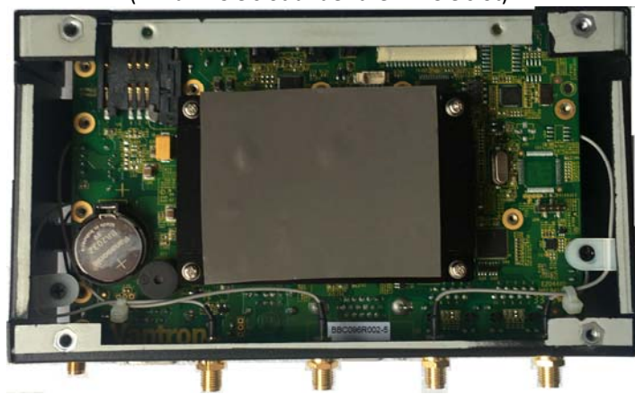
Top View for thermal module
